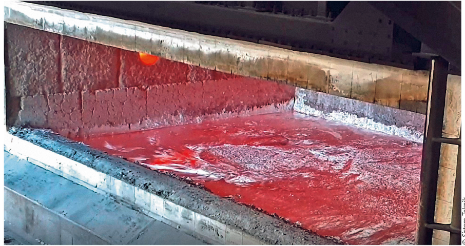
Stirring process in the aluminium bath by Sistem Teknik-designed electromagnetic stirrer
