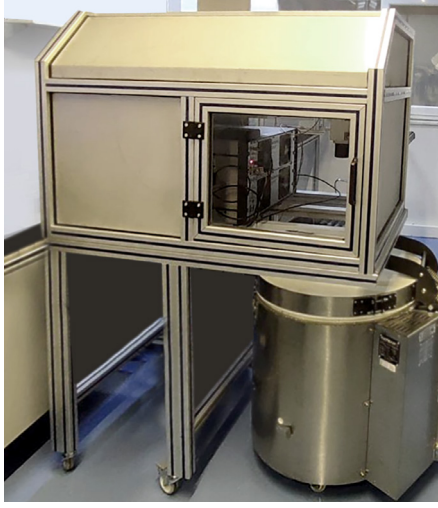
Figure-1 ST LIBS molten aluminum analysis prototype in the STAR Lab
